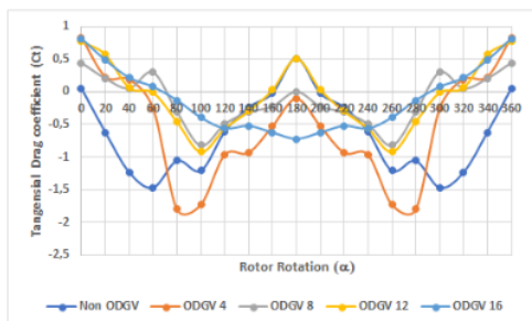
Figure 11. The tangential drag coefficient of the swirling savonius rotor at Re = 1.1 \times 10^5
